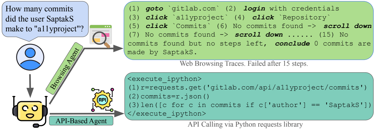
Figure 2: The API-Based Agent often solves problems in fewer steps than the Browsing Agent . In this task, web browsing failed to solve the intent “find the number of commits the user SaptakS made to the repo a1lyproject ” after 15 steps, while the API-Based Agent successfully completed the task with only three lines of code.
