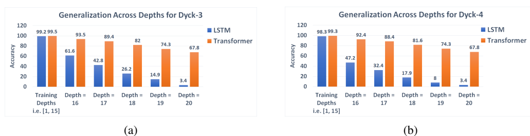
Figure 4: Generalization of LSTMs and Transformers on higher depths for (a) Dyck-3 and (b) Dyck-4. The lengths of strings in the training set and all validation sets were fixed to lie between 2 to 100.
