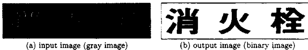
Figure 4: A result of the binarization using (Otsu 79) method
