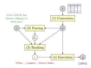
Figure 2: The prediction framework: (1) the table t is deterministically converted into a knowledge graph w as shown in Figure 3; (2) with information from w, the question x is parsed into candidate logical forms in  $Z_x$ ; (3) the highest-scoring candidate  $z \in Z_x$  is chosen; and (4) z is executed on w, yielding the answer y.
