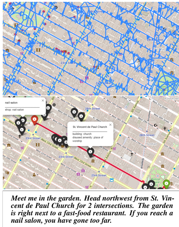
Figure 1: Our method for generating spatial descriptions samples from the graph-map (top) a path (middle image, red line), a starting point (green marker), a goal point (red marker), and prominent landmarks (black markers). It then generates an instruction (bottom) from the spatial relations between these entities.
